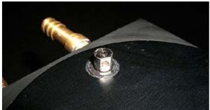
Fig. 3 Insertion of radiation rod in the fog chamber
