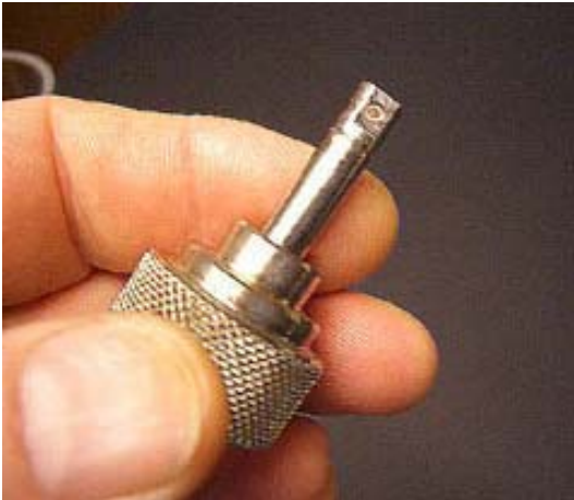
Fig. 3 Insertion of radiation rod in the fog chamber
