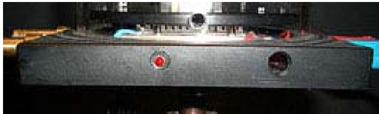
Fig. 4 Signal LED (overheating protection) and hole for temperature measurement
