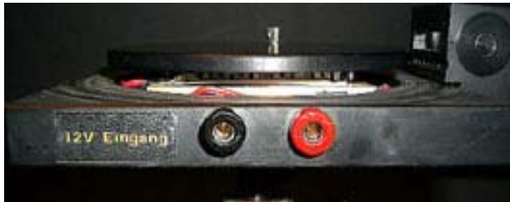
Fig. 5 Connections for supply voltage (12-15V / 8A)
