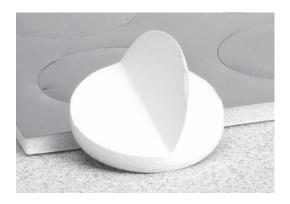
3. Place the Fast Response Temperature Probe sensing tip in the center of the disk adhesive.
