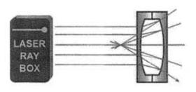
E19b Light beam passing through air convex lens
