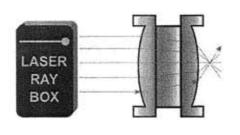
E18a Light beam passing through glass concave lens – the rays are parallel to the optical axis (RODS/RODS+)
