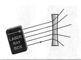
E19a Light beam passing through air convex lens – the rays are parallel to the optical axis (RODS+)
