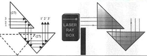
E11e Reflection of light on two glass prisms (RODS+)
