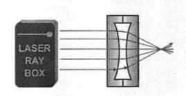
E20b Light beam passing through air concave lens – the rays are non-parallel to the optical axis (RODS+)
