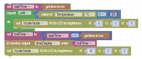
We can use the **get time in ms** block to get a timestamp of when an event happens. In our example we can use the block to determine how long it takes for the temperature to reach 25 °C. The time can be displayed using the **number output** block from the Code Output (on page 123) group.
