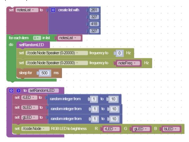
Functions are used to store repeatable tasks and make code easier to read. In this example, we have a function named <code>setRandomLED</code> that sets the //code.Node RGB LED to a random color. By putting this code in a separate function our main code block is easier to read.
