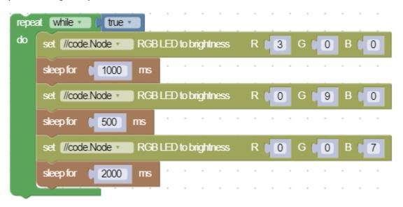
Sleep blocks pause the code for a designated amount of time. In this example, the red LED is turned on for one second, then the blue LED is turned on for a half second, and finally the green LED is turned on for two seconds. Note that when a program is sleeping it is not performing any other task.
