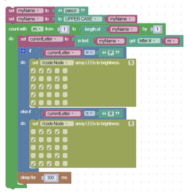
In this example the string "pasco" is changed to uppercase and displays the letters "P" and "S" on the //code.Node LED array.
