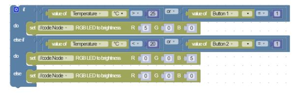
Adding to Example 3, if the temperature is less than 20 °C *or* Button 2 is pressed, the blue (B) LED will turn on. Otherwise, all the LEDs will turn off.
