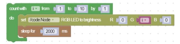
This loop will initially set the green LED's brightness to 1 and increment by 1 until 10 is reached. The LED will stay at each brightness level for 2 seconds.
