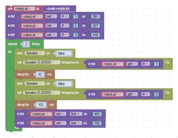
A variable can be set from a list of numbers one value at a time. In this example, a variable is set to a list containing three different integers. In the loop, the //code.Node speaker is set to play the frequencies of the #1 and #3 values in the list, change the first and last values of the list (which happen to be #1 and 3), and play those values again. The speaker output will sound different than the first round because we changed the frequencies after going through the loop one time.
