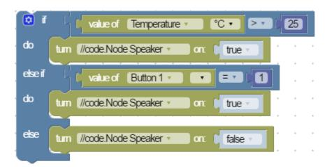
This example uses **else if** and **else** statements. If the temperature is less than 25 °C but Button 1 is pressed, the speaker will still turn on. If neither scenario is true then the speaker will be turned off.
