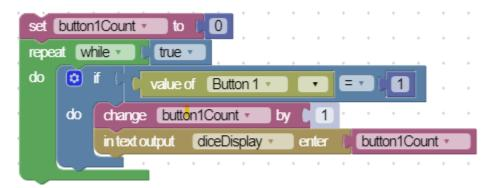
If a variable is a number, the **change by** block can be used to increase or decrease the value of the variable. In this example, the variable button1count increases by 1 each time Button 1 on the //code.Node is pressed.
