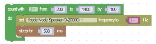
This loop will start the speaker at a frequency of 200 Hz and in increase by 100 Hz until the loop reaches 1400 Hz. Each frequency will be played for 0.5 seconds.
