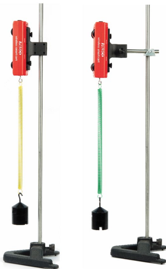
Figure 2. The Smart Cart can be mounted directly to a vertical rod (left) or to a horizontal cross-rod (right).
