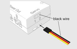
The //control.Node On-board Sensor can measure the servo current. You can use this measurement to detect a resisting force when the servo is trying to maintain a specified position. The Servo Current increases in response to resisting the force.
