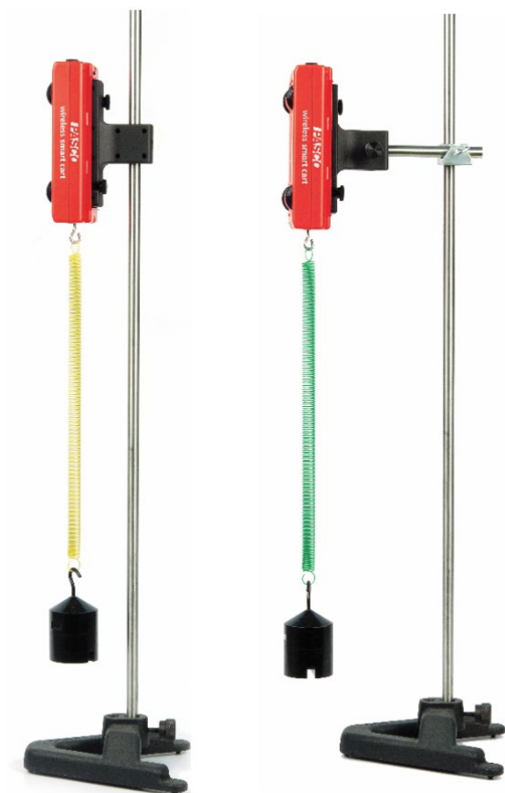
Figure 2. The Smart Cart can be mounted directly to a vertical rod (left) or to a horizontal cross-rod (right).
